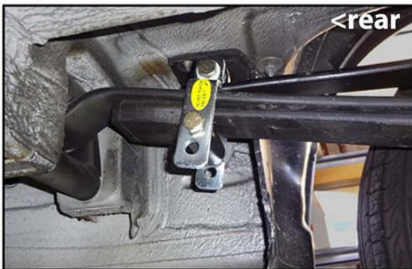
Install rear shackle in the upper bolt position
