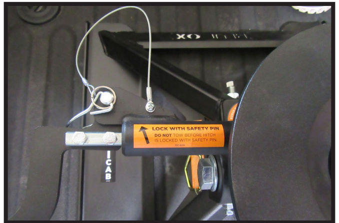
4. Once hitch is hooked up to the king pin of the trailer, turn handle and reinstall locking pin.
