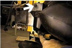
13. Remove three metric bolts from windshield washer reservoir on driver's side. Using the phillips screw driver, remove screw from tubing on reservoir and set aside.
