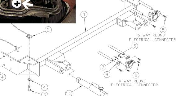
**IMPORTANT:** Use only genuine factory replacement parts on your Base Plate. Do not substitute homemade or nontypical parts. If a bolt is lost or in need of replacement, for your safety and the preservation of your Base Plate, be sure to use a replacement bolt of the same grade (Usually Grade 5, refer to parts list). Repair parts may be ordered through your nearest **Blue Ox** dealer or distributor.
