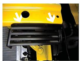
11. Remove two christmas tree clips on lower grill just under metal bumper, set lower grill insert aside. Lower grill insert will NOT be reinstalled.
