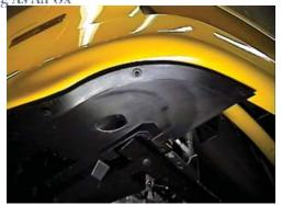
7. Remove the three metric bolts just forward of the front tire, on the bottom side of fascia, both sides.
