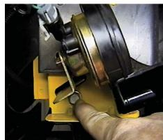
**12.** Using the 13MM socket, remove metric bolt from horn bracket and set aside.
