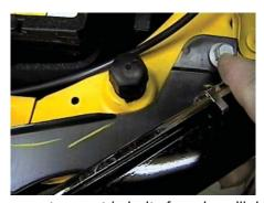
3. Remove two metric bolts from headlight assembly with the 10MM socket, pull forward, unplug electrical and set aside, both sides.
