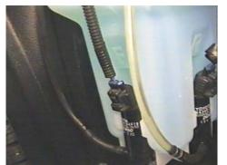
5. Disconnect tubing and plug. Disconnect electrical couplers.
