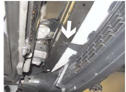
**4.** On the bottom of metal bumper, behind fascia, remove one push pin from fascia tab, both sides. Pull fascia forward and set aside.
