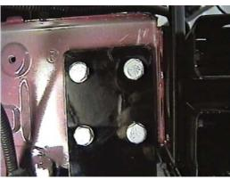
9. Using the baseplate as a template, drill four holes with the 13/32" drill bit, both sides. Insert item 2 into 1 1/4" hole, to align with drilled holes on the inside of frame. Tighten items 3 and 4 into item 2 on the four 13/32" drilled holes, both sides. Be sure and use loctite on all bolts before tightening.
