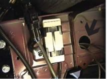
**7.** Using either a 1 1/4" drill bit or hole saw, drill a 1 1/4" hole in frame, to gain access to inside of frame. both sides.
