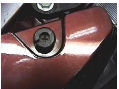
Remove phillips screw with rubber bumper using the phillips screw driver, both sides. On the top side of front fascia, remove three phillips push pins and two push pins from upper fascia opening.
