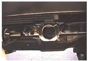
Hold baseplate in place. Temporarily clamp baseplate to the bottom side of metal bumper, while holding a 3/4" space between the bottom of metal bumper and cross tube.
