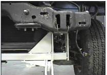
Install Base Plate according to assembly drawing on last page.
