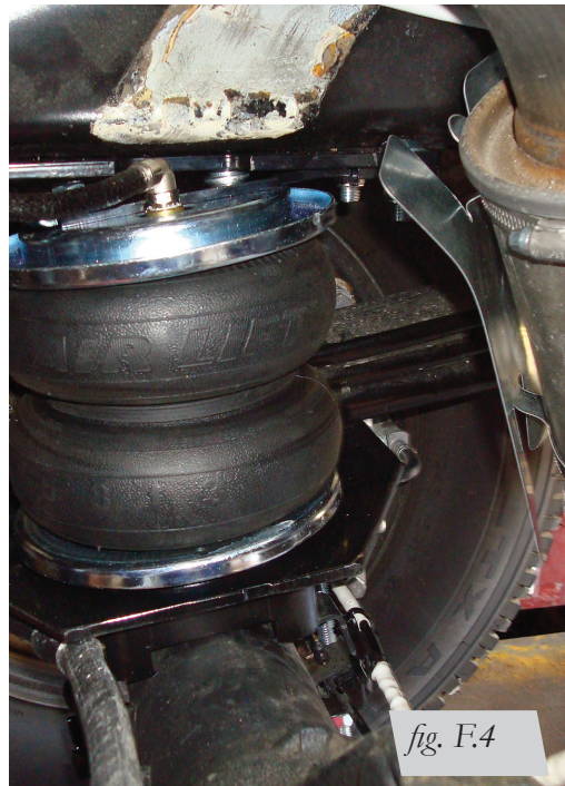
Passenger's (right) side inside frame view of kit installed.
